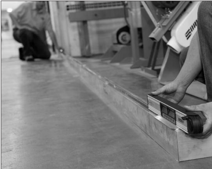
Align the "PAL" Tool with Base Shoe and point toward the Laser Target set at opposite end.
